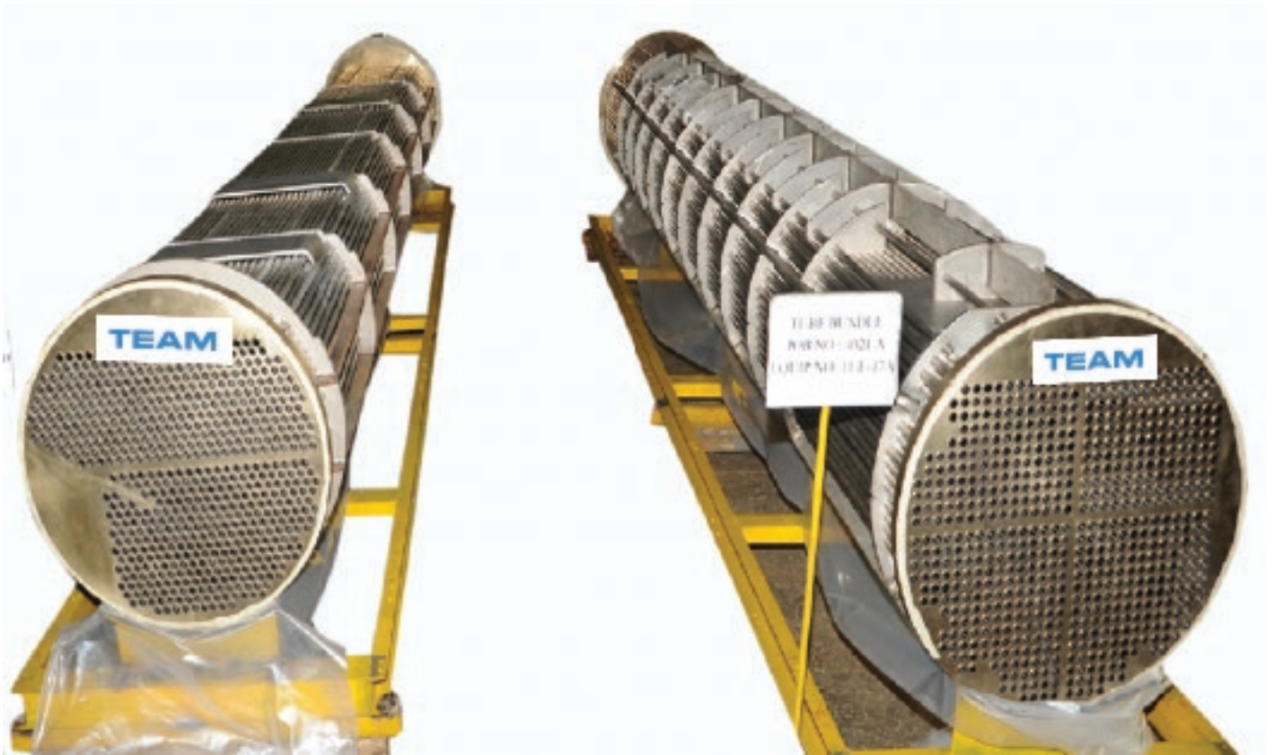
CLIENT : HPCL EQPT. : HEAT EXCHANGER TUBE BUNDLE MOC : TITANIUM TUBE + NAB TUBESHEET
