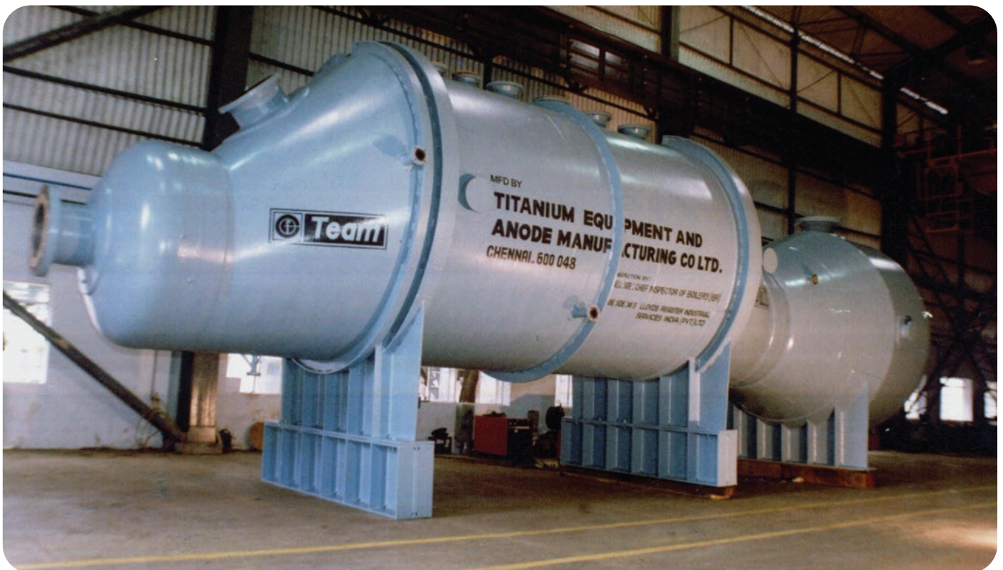
CLIENT : RIL - PATALGANGA EQPT. : ELP STEAM RAISER MOC : CS + Titanium Cladded Heat Exchanger
